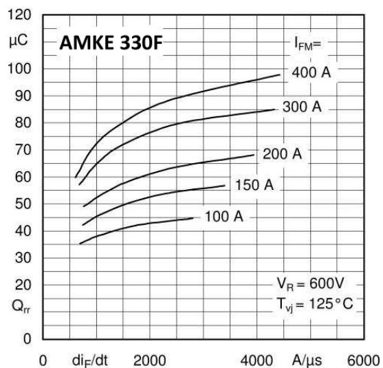
Fig. 1 Typ. recovery charge vs. current decrease
