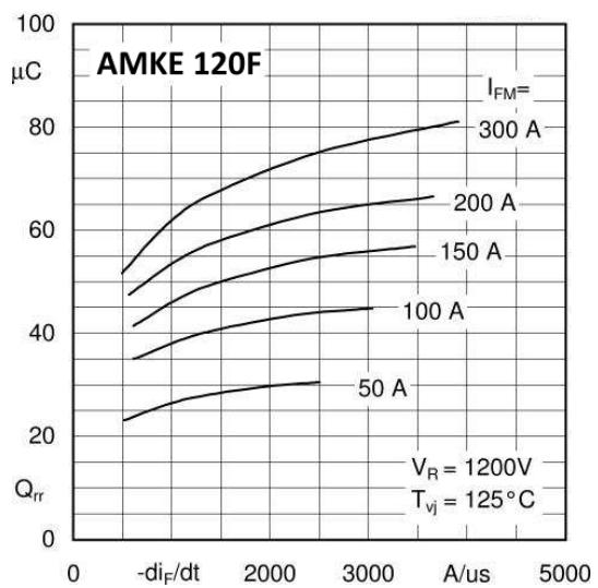
Fig. 1 Typ. recovery charge vs. current decrease
