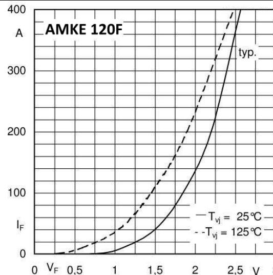
Fig. 4 Typ. forward characteristics
