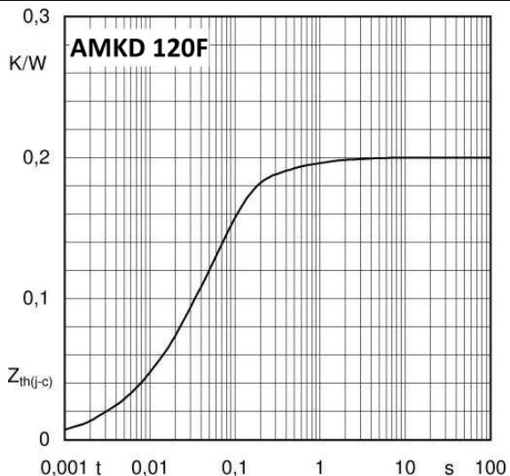
Fig. 3 Transient thermal impedance vs. time
