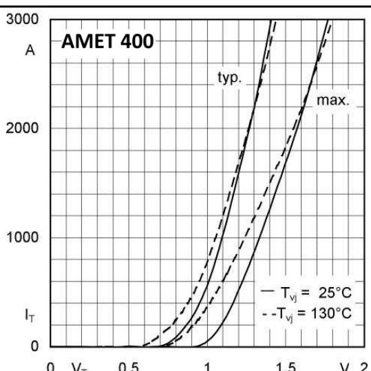
Fig. 7 On-state characteristics
